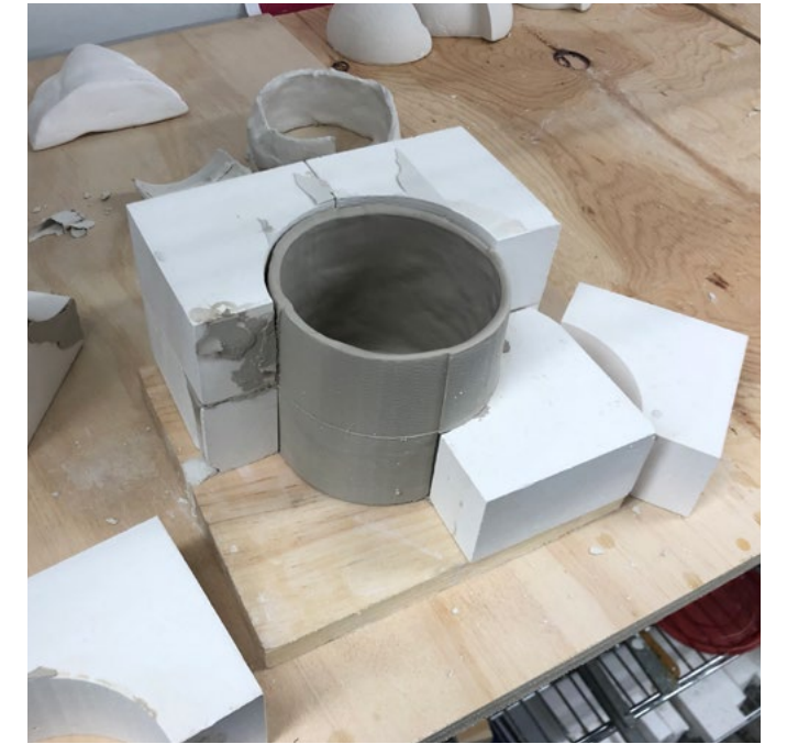
Slip Casting Process
